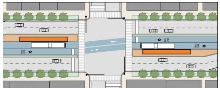
Alternative 1: Median-Running Dedicated Lanes and Station Location
